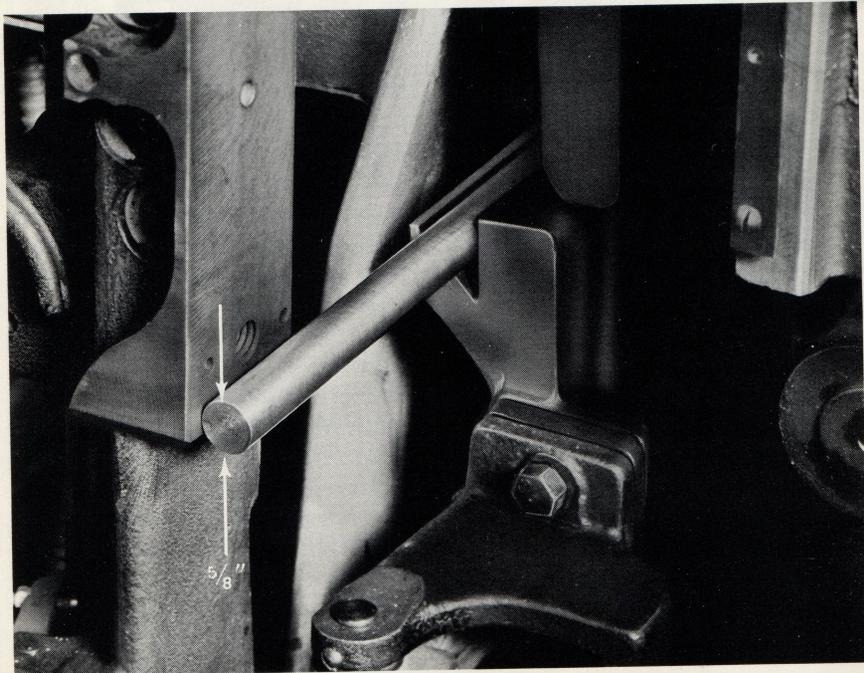
is fitted, drive the vise shaft back to the right far enough to remove the left hand bushing. Take a micrometer reading of the old bushing and lay it aside.
